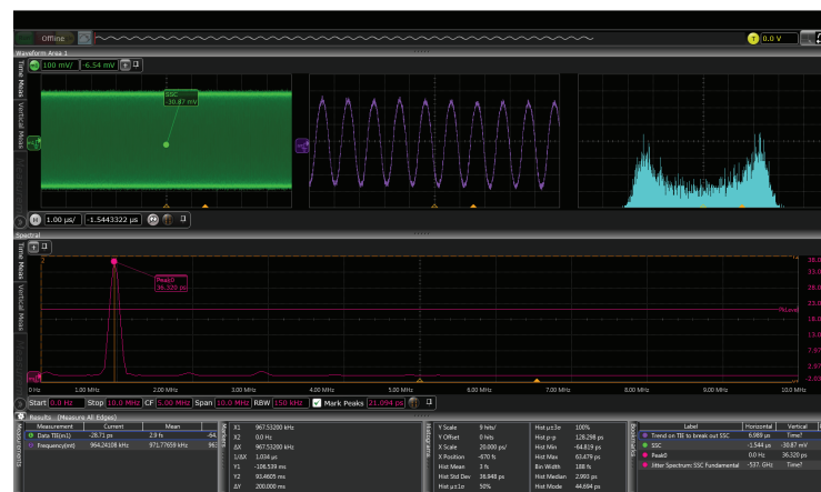
Figure 8. A spectrum display shows the spectral content of the jitter, useful for identifying sources of jitter by their frequency components.
