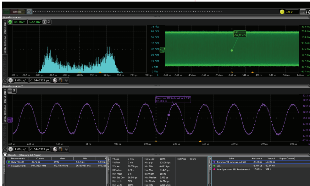
Figure 1. The software provides multiple views of jitter, including histogram, trend, and spectrum, for maximum insight
